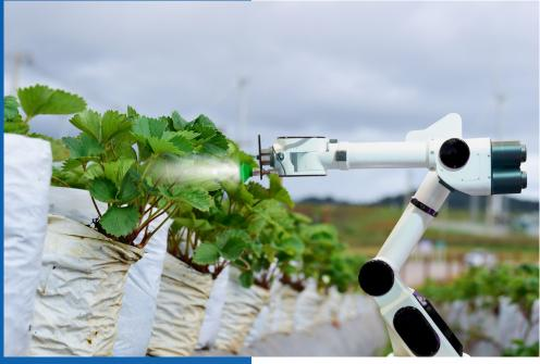
In particular, for sprayed chemicals, there is potential for challenges after the formulation droplet exits the machine. Spray drift may not always be easy to predict and model given real world, gusty or swirling wind conditions. After the droplet has landed, there are further potential challenges of splash back and the formation of ultrafine droplets which can be picked up by the wind and uncontrollably spread through the field and the
