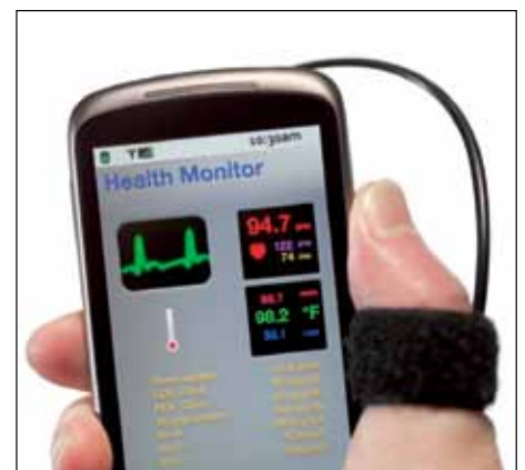
Handheld device records ECG data for remote review by clinician.
